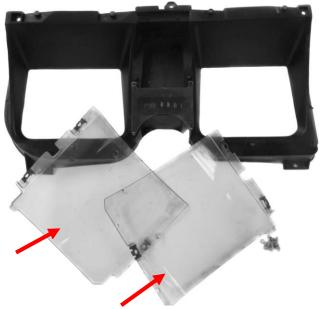
5. This step is optional for automatic transmission bezels only. If you purchased a separate GSS universal gear kit from Dakota Digital, the gear position can be displayed in the HDX message centers; therefore the stock gear position indicator can be removed.
